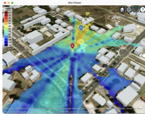
Figure 35: Coverage with Antenna ITU-R M.2412 and 0 reflections.
