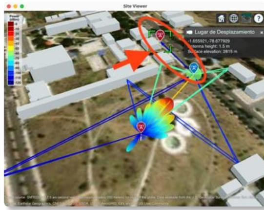
Figure 32: Ray tracing and visualization of the place of displacement of the receiver.
