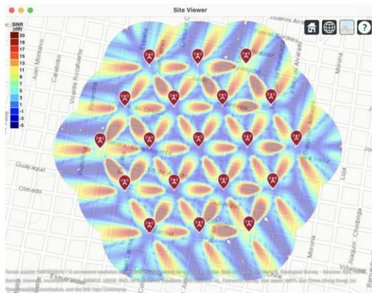
Figure 29: Top view of SINR map within a topographic map.
