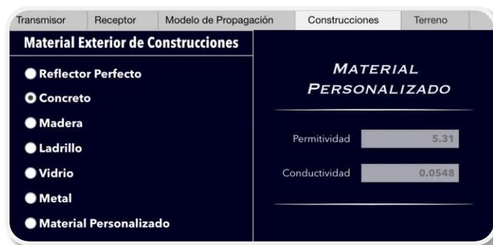
Figure 15: Parameter window for exterior materials in the parameterizable simulator.
