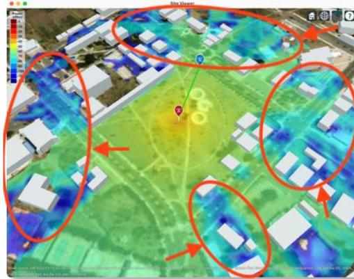
Figure 38: Coverage with an isotropic antenna with 10 reflections.
